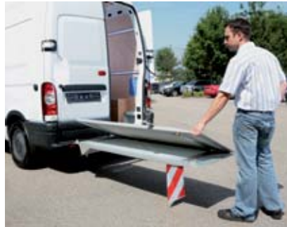
Open hydraulically and unfold by hand.
