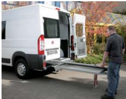
Open hydraulically and unfold by hand.
