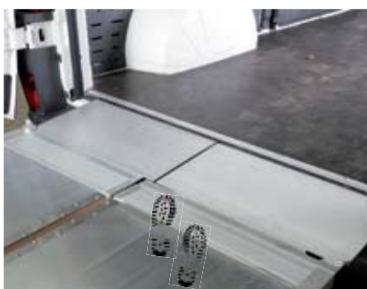
The two-part VanBridge connects the vehicle floor and the platform. Platform safety with TracGrip and SideGrip.
