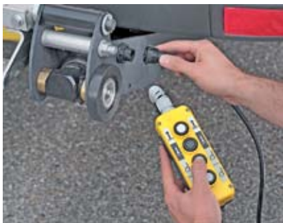
Emergency control unit.
