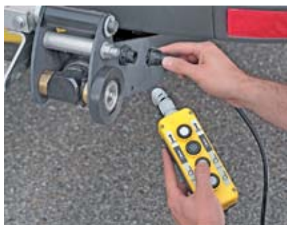
Emergency control unit.
