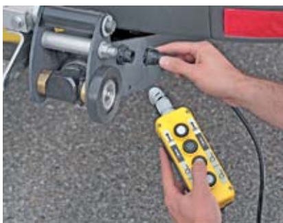
Emergency control unit.
