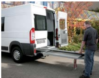
Open hydraulically and unfold by hand.
