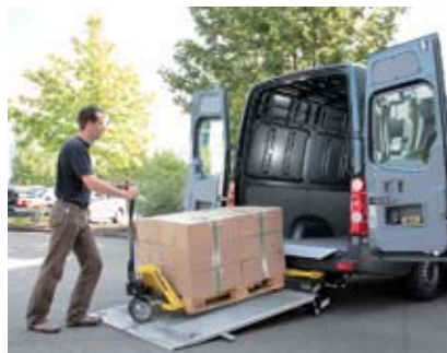
Enough room for euro pallets and lift trucks. Extremely low approach angle (6.2°). Please keep in mind pallet weight.
