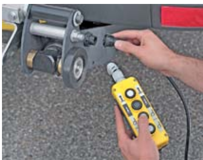
Emergency control unit.
