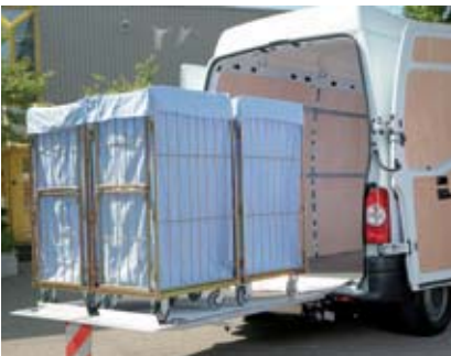
Standard: The trolley stop for 4 laundry trolleys or 1 foodstuffs trolley.
