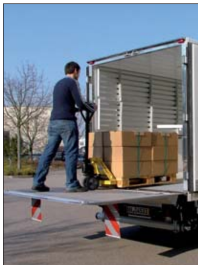
The BC 750S2 is stable and consequent also suitable for pallets. Platform safety with TracGrip and SideGrip.
