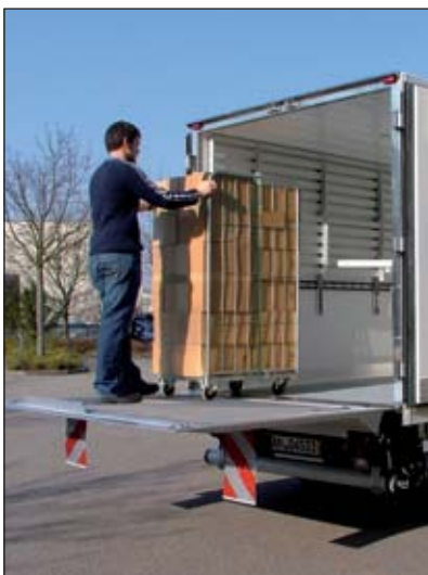
Efficient trolley transport with trolley stop 2ad or 2rd for two trolleys.
